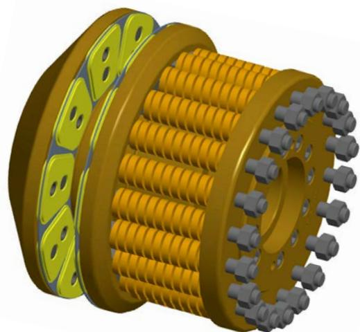
*In its RIMOSTAT® series, RINGSPANN realises a design principle that is essentially tailor-made for all applications where greater forces are at work. For here it is not disc springs but long ISO coil springs that, with a linear and flat curve progression, produce a contact pressure on the friction linings. (Image: RINGSPANN)*
