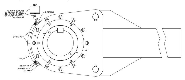
**Above:** Showing piping included for the configuration of visual gauge & breather.
